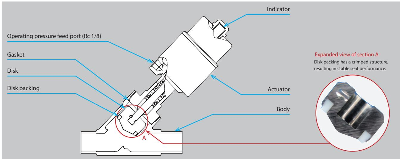
Actuator can turn 360°, allowing adjustment of orientation of operating pressure feed port.
