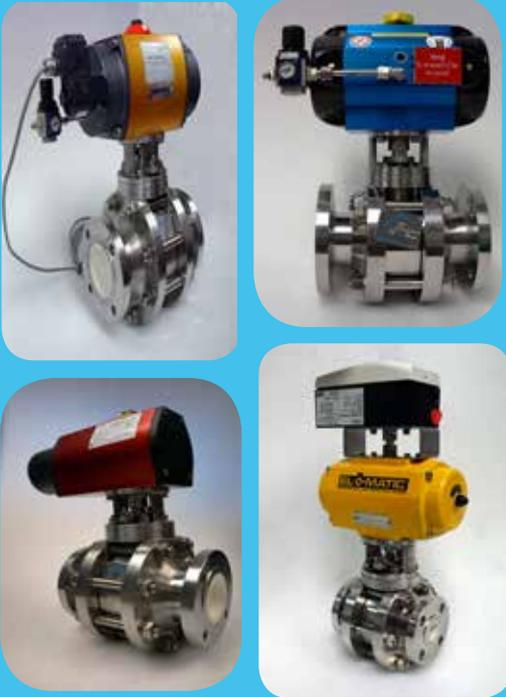
All Carten *HiLife* valves include a stainless steel bracket, or yoke interface, and coupling which meet the dimensional standards of ISO 5211 and provide a compact and direct fit onto most rotary actuator brands and models including electric and pneumatic. There are many different options for our top works including pressure reducing regulators, electro pneumatic positioners (smart, analogue), solenoid valves and limit switches.
