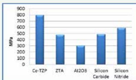
Figure 2: Fracture Toughness Comparison
