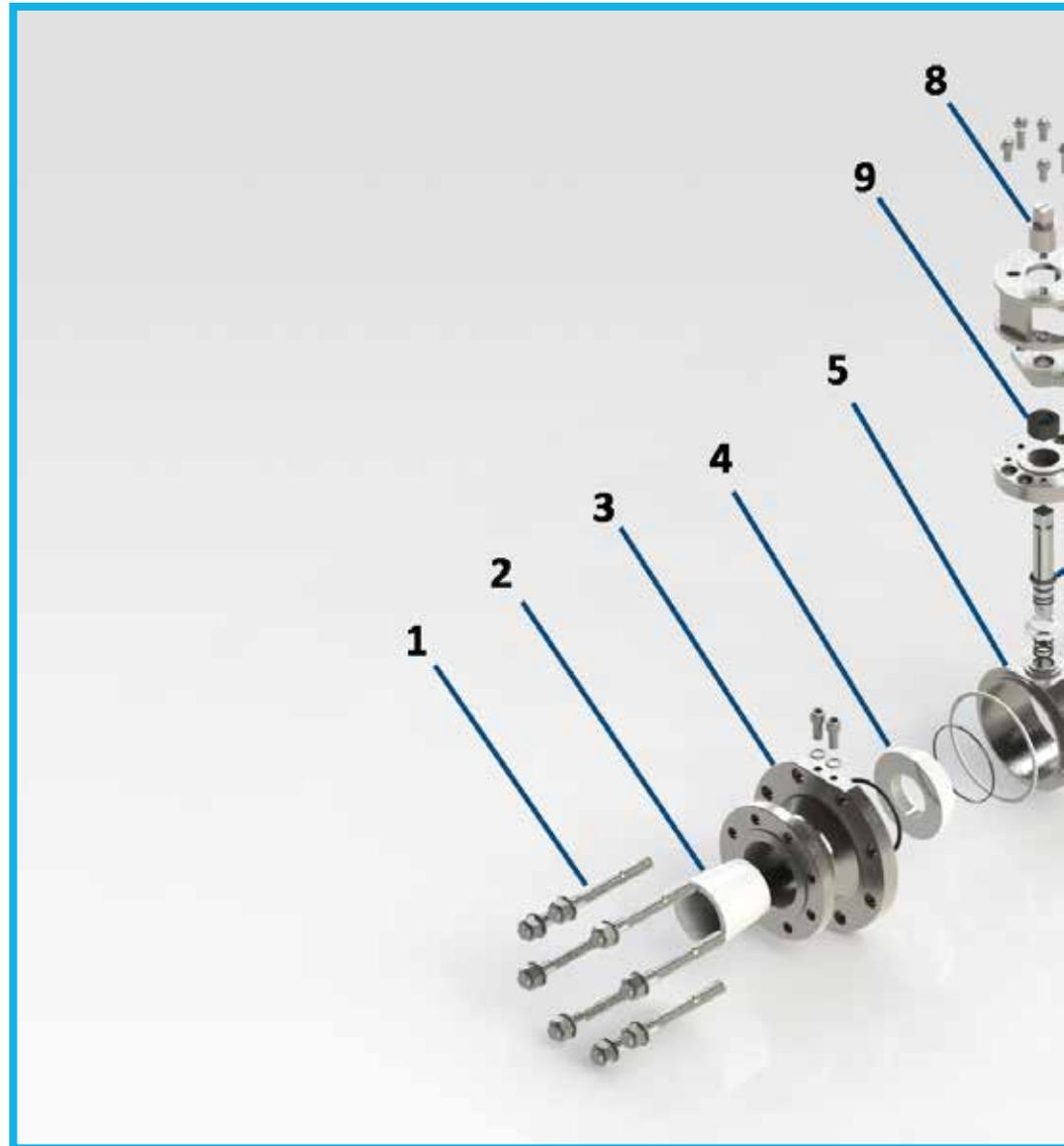
**6** Stainless Steel Bonnet Flange offers excellent corrosion-resistant properties and design strength to secure the appropriate leak-tightness specification, in addition to compressing against the machined one-piece hastelloy stem lip - therefore providing a blow-out proof design feature
